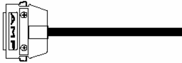
Figure 4-7: ECL/PECL I/O Card Pigtail Cable
