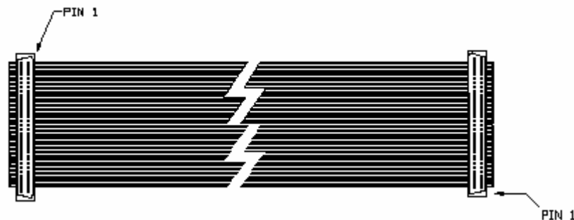
Figure 4-6: ECL/PECL I/O Card Ribbon Cable
