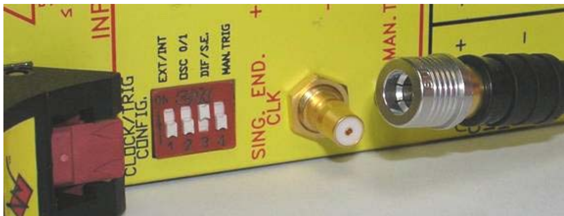
Figure 3-8: QMA Cable/Connector End (detail)
