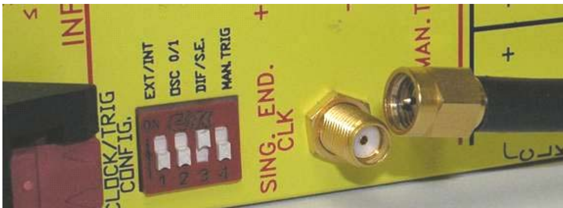
Figure 3-7: SMA Cable/Connector End (detail)
